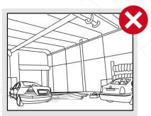
**No. Why?** There is no localised removal of exhaust fumes. General ventilation is inadequate to protect against exposure.
