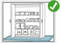
**Yes. Why?** The containers are labelled and arranged in a specific, ventilated and marked area, which has spill containment.
