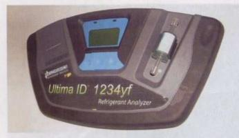
Handheld refrigerant identifiers for R-1234yf also identify R-134a and other refrigerants. They will have USB output to new recovery/recycle/recharge machines, which will operate only if the identifier sample from a vehicle system is R-1234yf, to prevent machine contamination.
