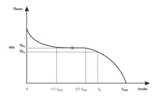
Th<sub>A</sub> = average thrust (the average thrust is determined by integrating the values between 1/3 and 2/3 of the total stroke  $S_{max}$ )
